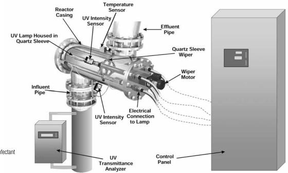
Fig. 1 — Example of UV disinfectant equipment (EPA Guide 2006)
