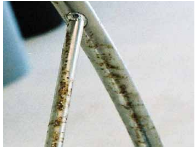
Figure 4: This chrome plated carbon steel reel for holding lane markers has only been in use for a few years but there has already been substantial corrosion under the plating. Photo Courtesy of TMR Consulting.
