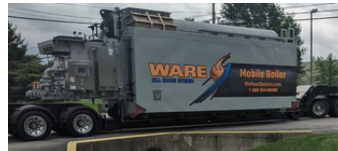
Trailer Mounted Rental Boilers
